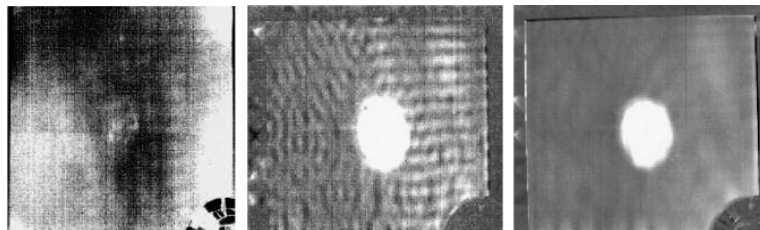
FIGURE 9. Three kinds of ultrasound thermography performed on the same local thermal damage in a CFRP-plate. Left: one image taken from the recorded temperature sequence 0.52 s after ultrasound burst (maximum thermal contrast), middle: monofrequent excitation f_R = 20 kHz, phase evaluation at 0.06 Hz, right: frequency modulated excitation ( f_R = 17 \dots 23 kHz, f_{\text{mod}} = 25 Hz), phase evaluation at 0.06 Hz.
