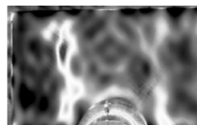
d) Ultrasound Lockin Phase image at 0.01 Hz, 400 W, and 100 seconds acquisition time
